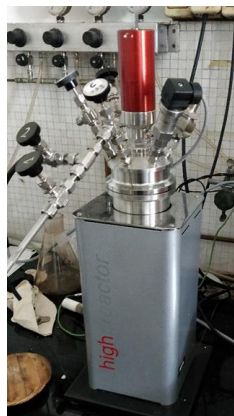
Figure 1: Berghof high pressure reactor (BTC-3000, Germany) used for the autohydrolysis of wheat straw
