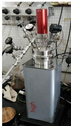
**Figure 1:** Berghof high pressure reactor (BTC-3000, Germany) used for the autohydrolysis of wheat straw
