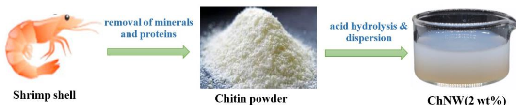
Figure 1: Schematic diagram of isolation of ChNWs from shrimp shell waste
