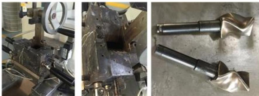
**Figure 1:** Lab scale mixing equipment
